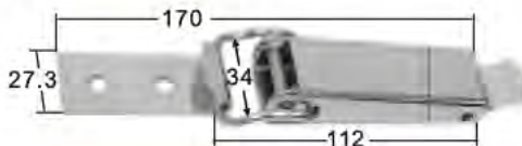
ECCENTRIC LATCH stamped AISI 304 ITEM NO. Thickness Weight 008358 2mm 180g
